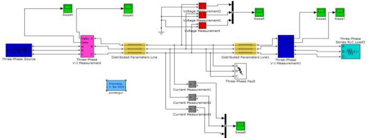
In the above figure-2 three phases Voltage-current (V-I) measurement blocks is used to measure V & I sample at source end. The transmission line is one line 100 Km long. Simulation of three phase fault simulator is used to simulate various types of fault. In transmission line faults are classified as L-G fault, LL-G fault and three phase fault.
