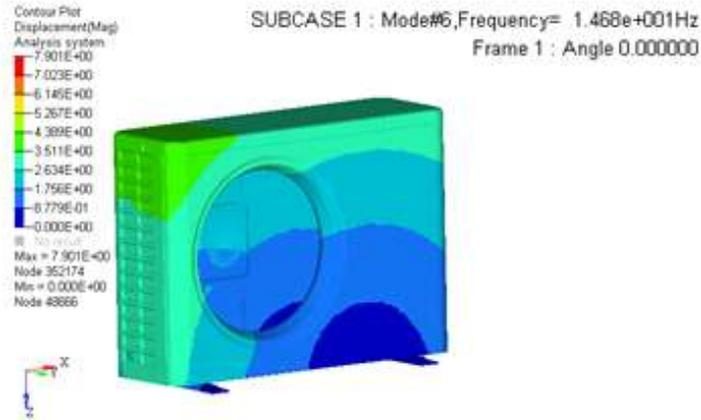
Figure 4: Mode shape for 6<sup>th</sup> mode of vibration ( $f_2=14.682\text{Hz}$ )
