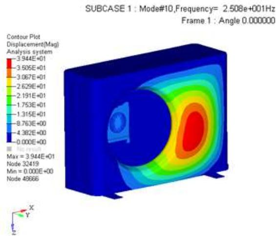
Figure 5: Mode shape for 10<sup>th</sup> mode of vibration ( $f_{10}=25.083\text{ Hz}$ )
