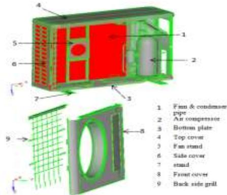
**Figure 1: Three Dimensional Model and different parts**
