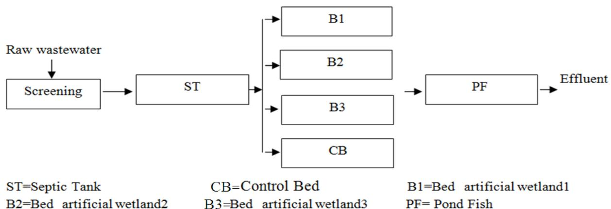
Figure 2. Schematic flow diagram for artificial wetland
