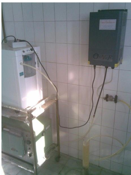
**Figure 3.** Ozone generator unit with generation power of 5 g/hr
