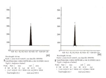
Figure 2: HPTLC Chromatogram of standard strychnine and brucine.
