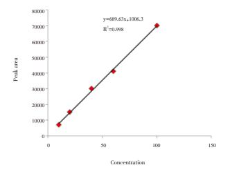
Figure 4: HPTLC calibration curve of standard strychnine.
