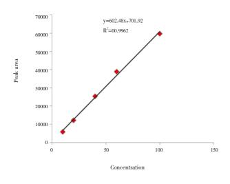
Figure 5: HPTLC calibration curve of standard brucine.
