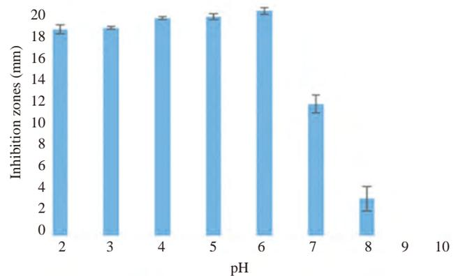
Figure 8. Activity of SCS of the LbM2a strain in different range of pH using *M. luteus* ATCC 10420 as indicator strain.
