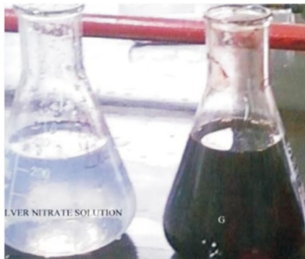
Figure 1. The reduction of silver nitrate to silver nanoparticles by addition of mushroom extract.
