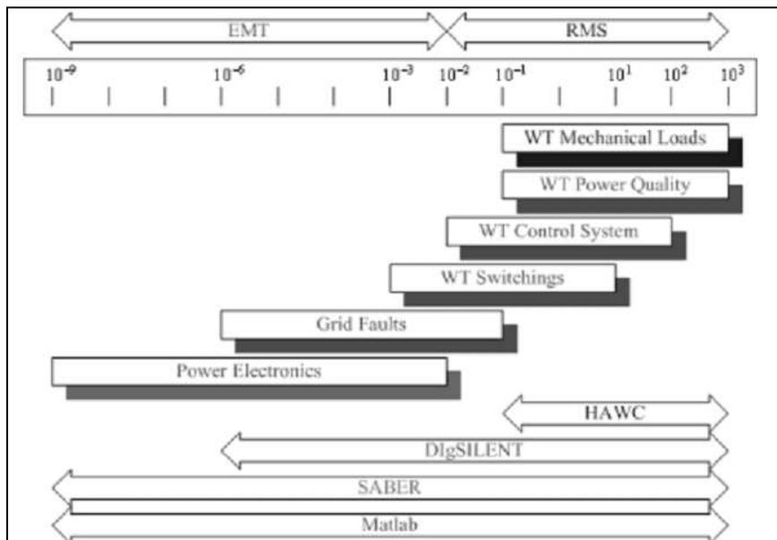
**Figure-4** Modeling aspects and levels in a WECS [33].
