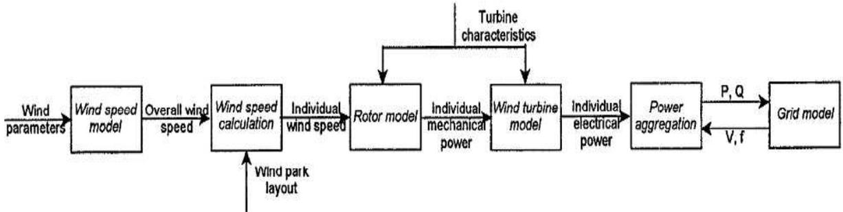
**Figure-3** Structure of aggregated model of wind park with variable speed wind turbines [3].
