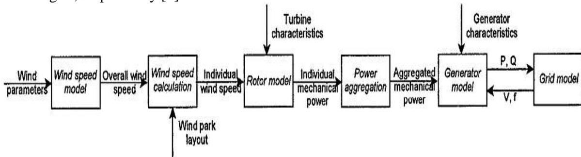
**Figure-2** Structure of aggregated model of wind park with constant speed wind turbines [3].
