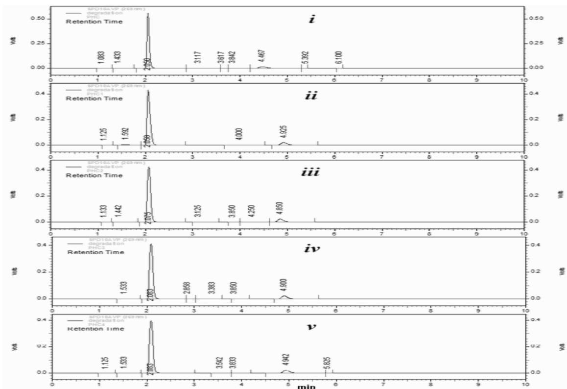
Fig. 6: HPLC chromatogram of 5-FU solution for their degradation under different pH after 24 h of storage at 1.2 (i); at 3.2 (ii); at 4.2 (iii); at 6.8 (iv), and at 6.8 (v)
