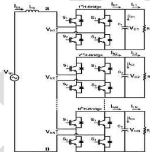
Fig. 3 Bidirectional CHB rectifier with N H-bridge cells.
