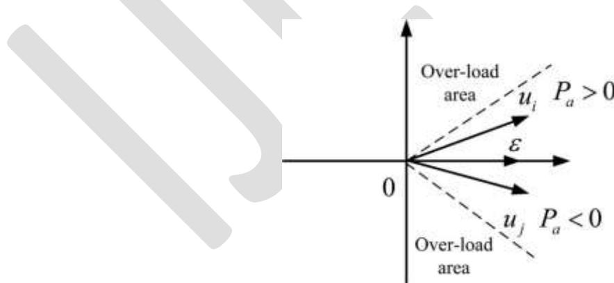
**Fig. 5** Output power control by phase adjustment.
