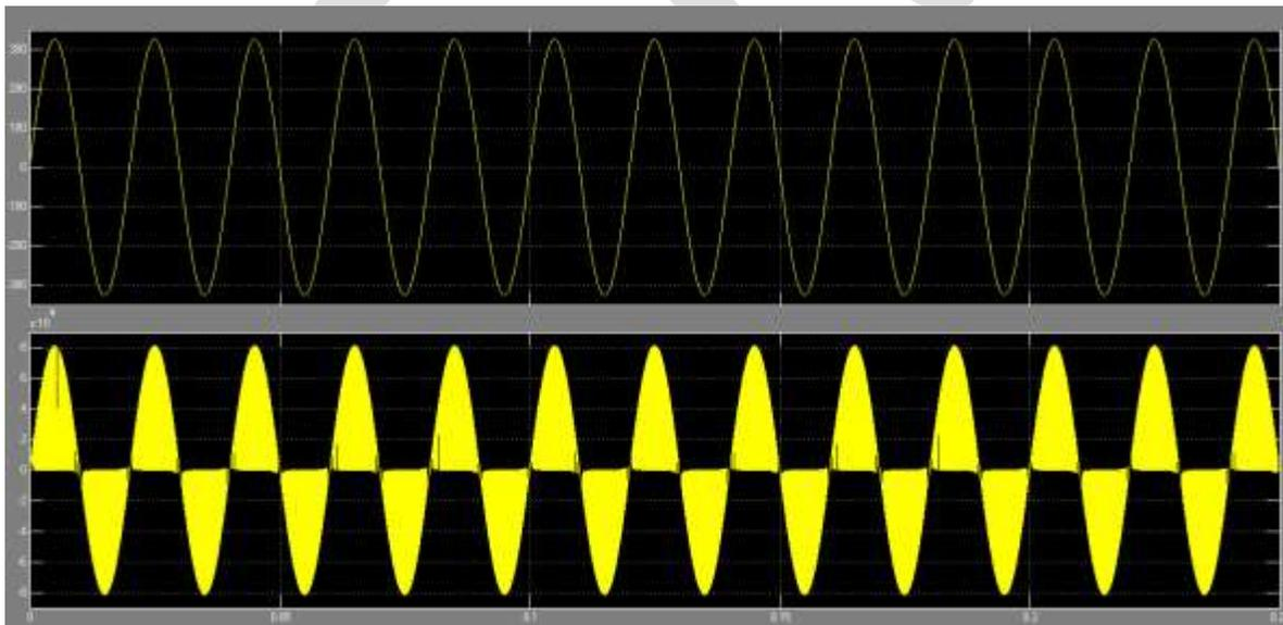
**Fig.8** Input voltage and current
