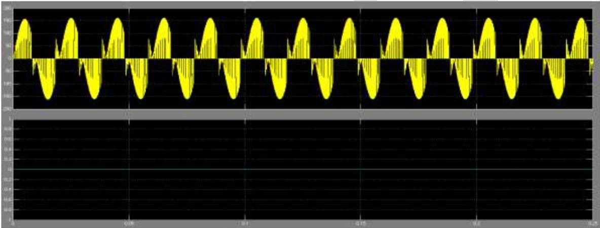
**Fig.10** Output voltage and current at no load
