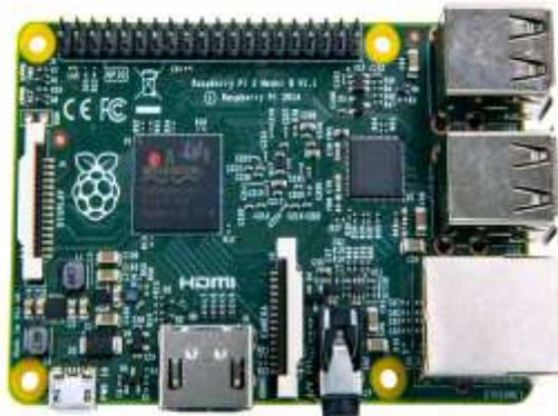
Fig.3: Raspberry pi board
