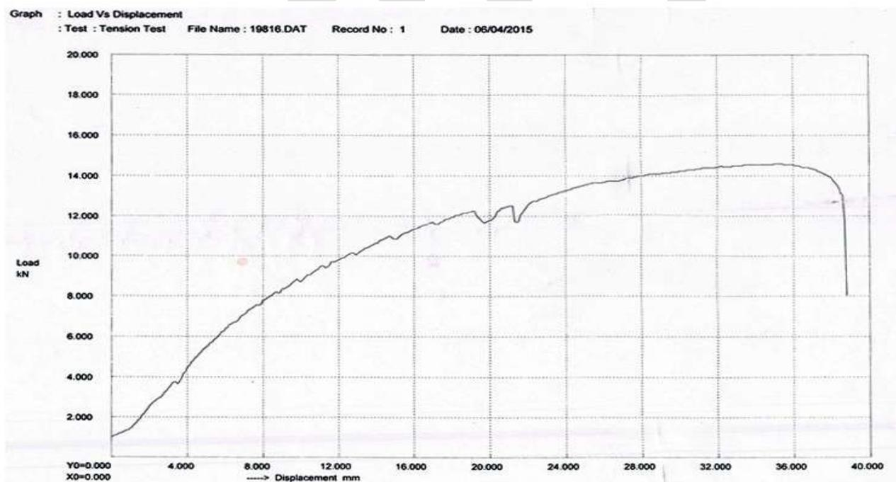
**Figure 5:** Stress v/s Displacement Graph for Sample 1
