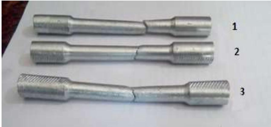
**Figure 4:** Tested specimen for tensile and elongation test
