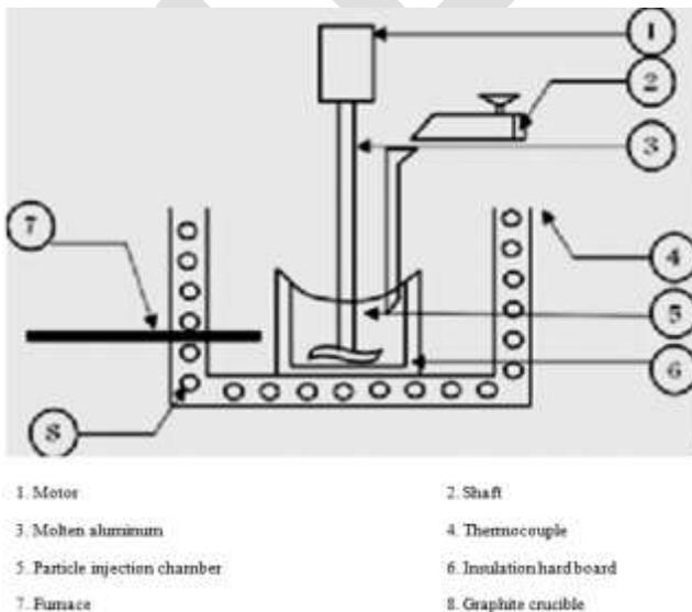
**Figure 1:** Schematic view of the Furnace [12]
