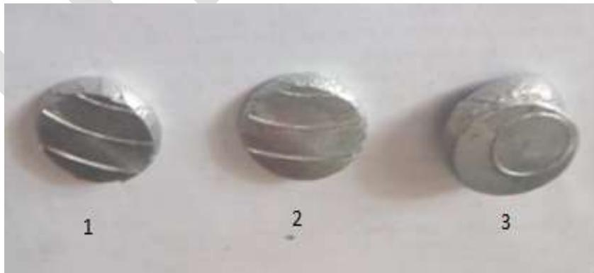
**Figure 9:** Tested specimen of Hardness Test
