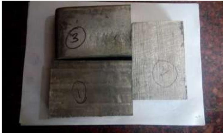
Figure 3: Fabricated Samples of AMC.
