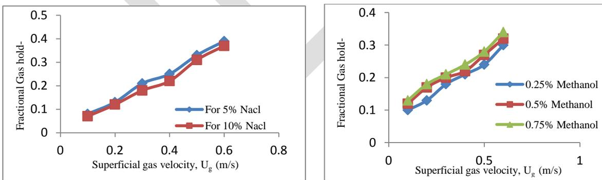
**Figure 3.4.1 Effect of superficial gas velocity on fractional gas hold-up by varying concentration of electrolyte (NaCl) and solvent ( $\text{CH}_3\text{OH}$ )**
