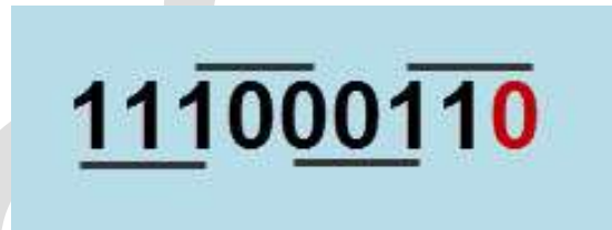
FIG 1.Bit Pairing as per Booth Recoding
