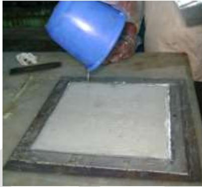
**Fig -2:** Pouring of Epoxy Resin
