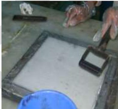
**Fig -3:** Removal of Entrapped Air by Rollers
