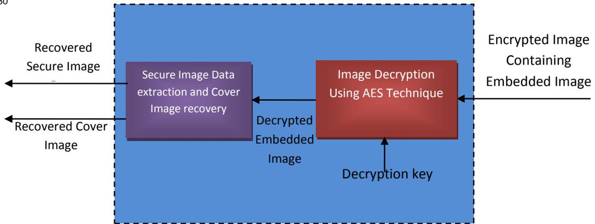
FIGURE (4) PROPOSED SECURE IMAGE DATA EXTRACTION SYSTEM
