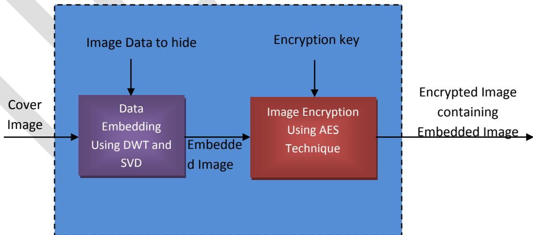
FIGURE (3) PROPOSED SECURE IMAGE DATA HIDING SYSTEM
