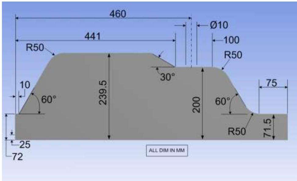
Figure 2: Combustor Dimensions
