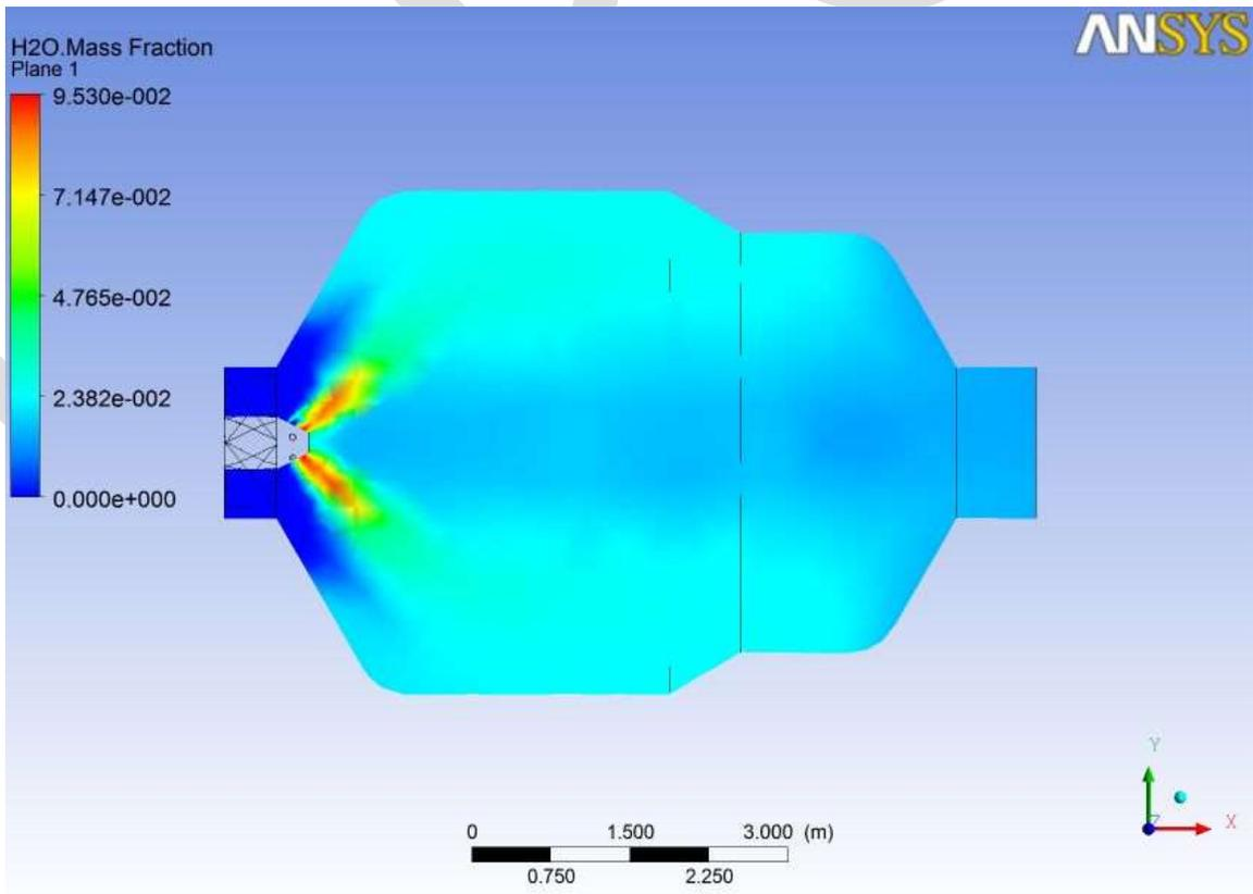
Figure 7:H<sub>2</sub>O Mass Fraction
