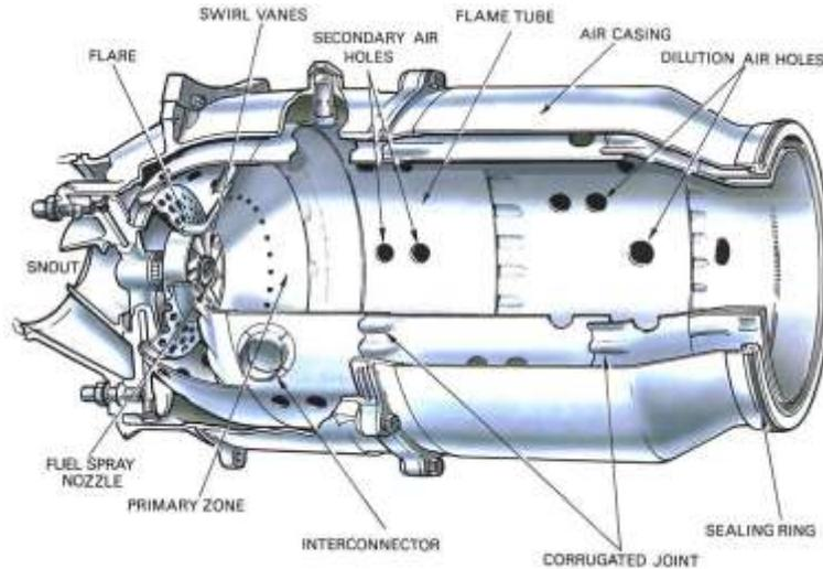
Figure 1: Can combustor
