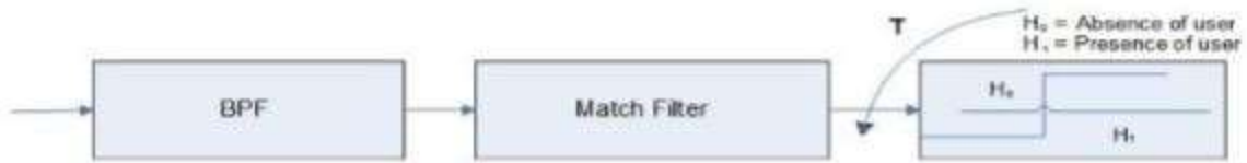
Fig 2: Block diagram of Matched Filter Detection
