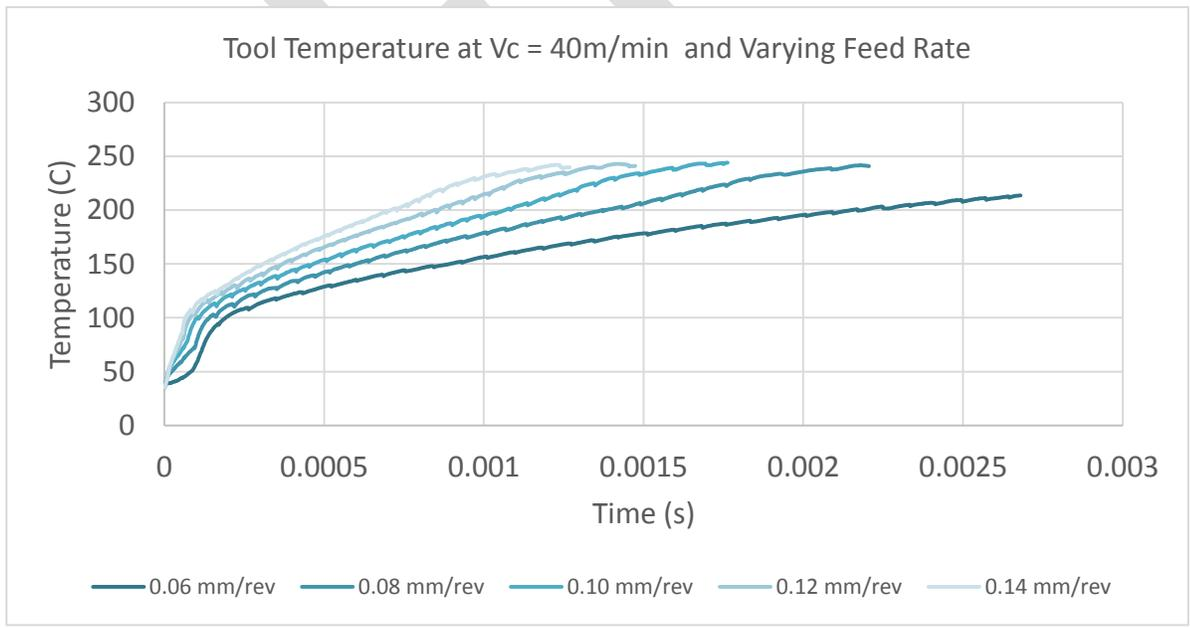
Fig. 5: Tool temperature at constant cutting velocity and varying feed rate
