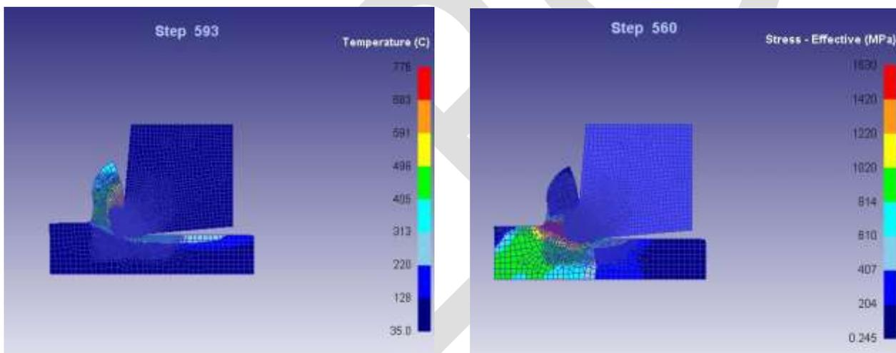
Fig. 2: a) Temperature Profile, b) Effective Stress Map developed using theoretical model at  $V_c = 40\text{m/min}$  and Feed Rate =  $0.12\text{ mm/rev}$
