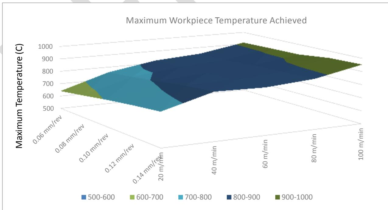
Fig. 8: 3D Plot showing the variation of Maximum Work-piece temperature with Cutting Velocity and Feed Rate
