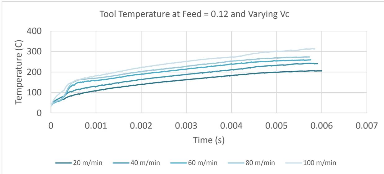
Fig. 6: Tool temperature at constant feed rate and varying cutting velocity
