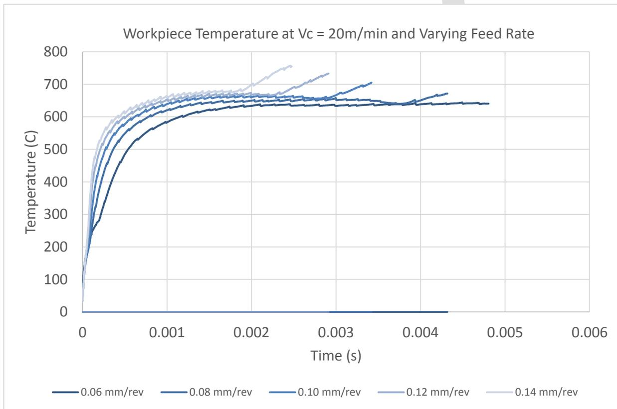
Fig. 3: Workpiece temperature at constant cutting velocity and varying feed rate
