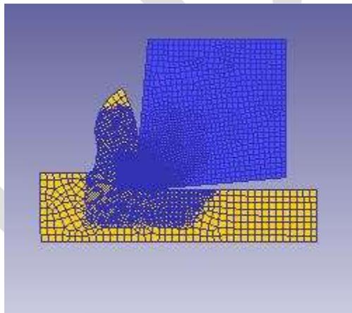
Fig.1: Simulation in Progress in DEFORM 2D
