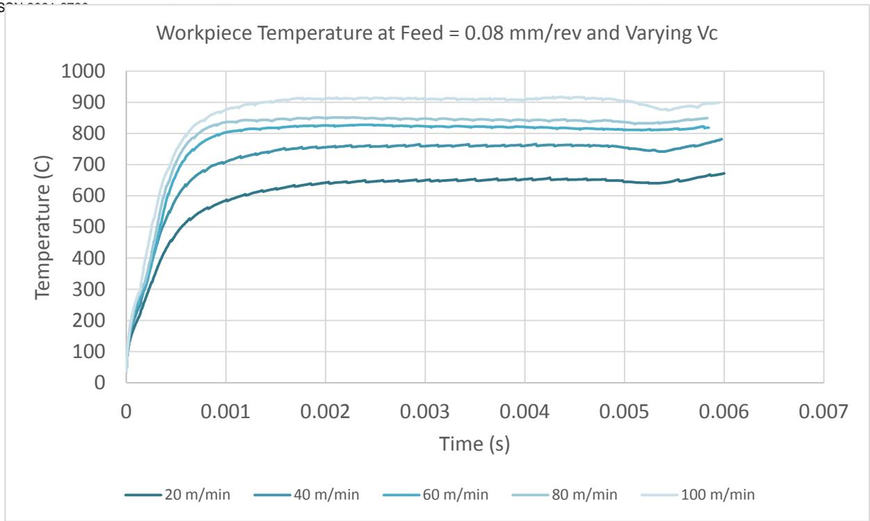
Fig. 4: Workpiece temperature for varying cutting velocity and at a constant feed rate
