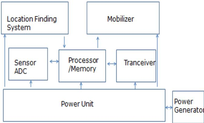
Figure 2. Components of a Sensor Node
