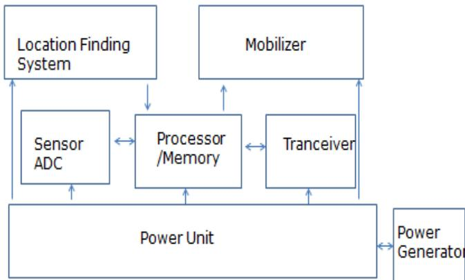
Figure 2. Components of a Sensor Node
