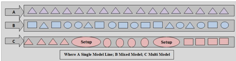
Figure 2. Assembly Lines for Single and Multiple Products (Becker and Scholl, 2003)
