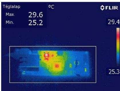
Fig. 3. Thermographic image about the controller panel of the DSN-PC board. The heat generator parts ( $\mu C$  and power supply) are clearly noticeable.
