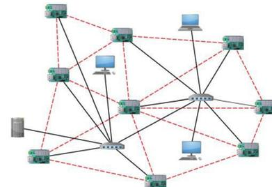
Fig. 1. The conception of DSN-PC sensor network, which forms the necessary grid for numerical calculations by using the nodes of the networked sensor stations not only for measurements and collection of data but for communication with their close and distant neighbors through the Internet and solve numerical weather prediction calculations by the Finite Difference Method (FDM) on a rectangular grid (a./) or by the Finite Elements Method (FEM) on irregular grid (b./) [2].
