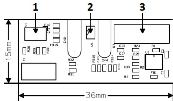
Fig. 5. Schematic of the separated sensor board with separated sensors on it. 1: MPL3115A2 barometer. 2: MCP9808 thermometer. 3: HIH-5031 relative humidity sensor.
