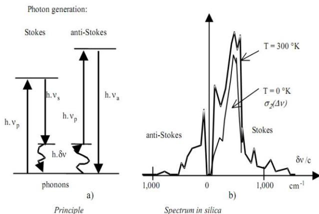
Fig. 1. Raman scattering: a) principle, b) spectrum in silica [2].
