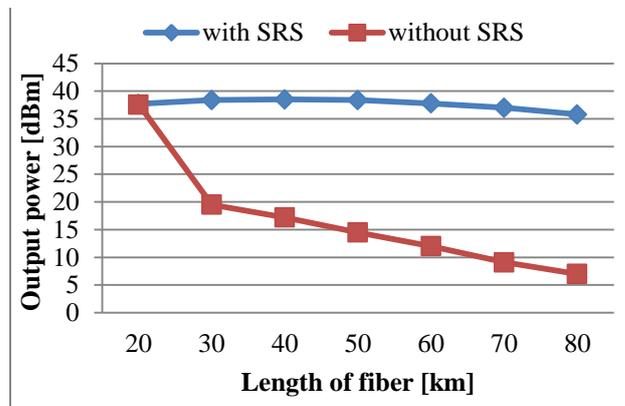
Fig. 4. The dependency of the output power on length of the fiber.
