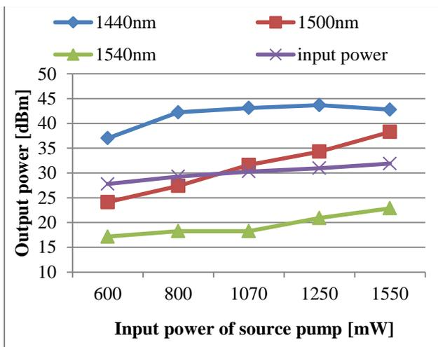
Fig. 5. Dependency of output power on position and power of source pump.
