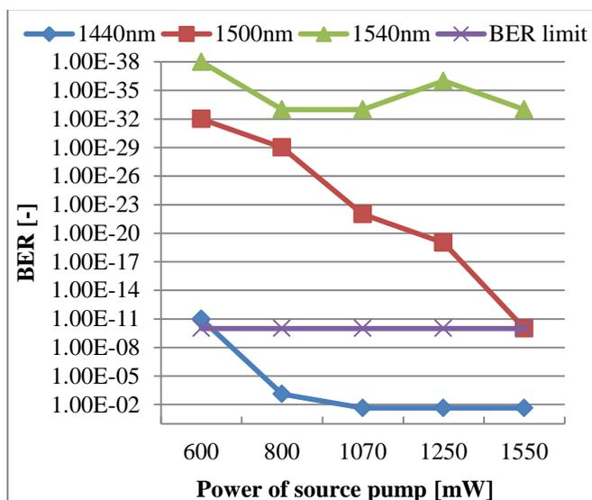
Fig. 6. Dependency BER on position and power of source pump.
