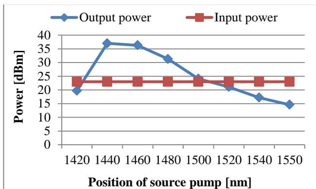
Fig. 3. Interdependency between input and output power.
