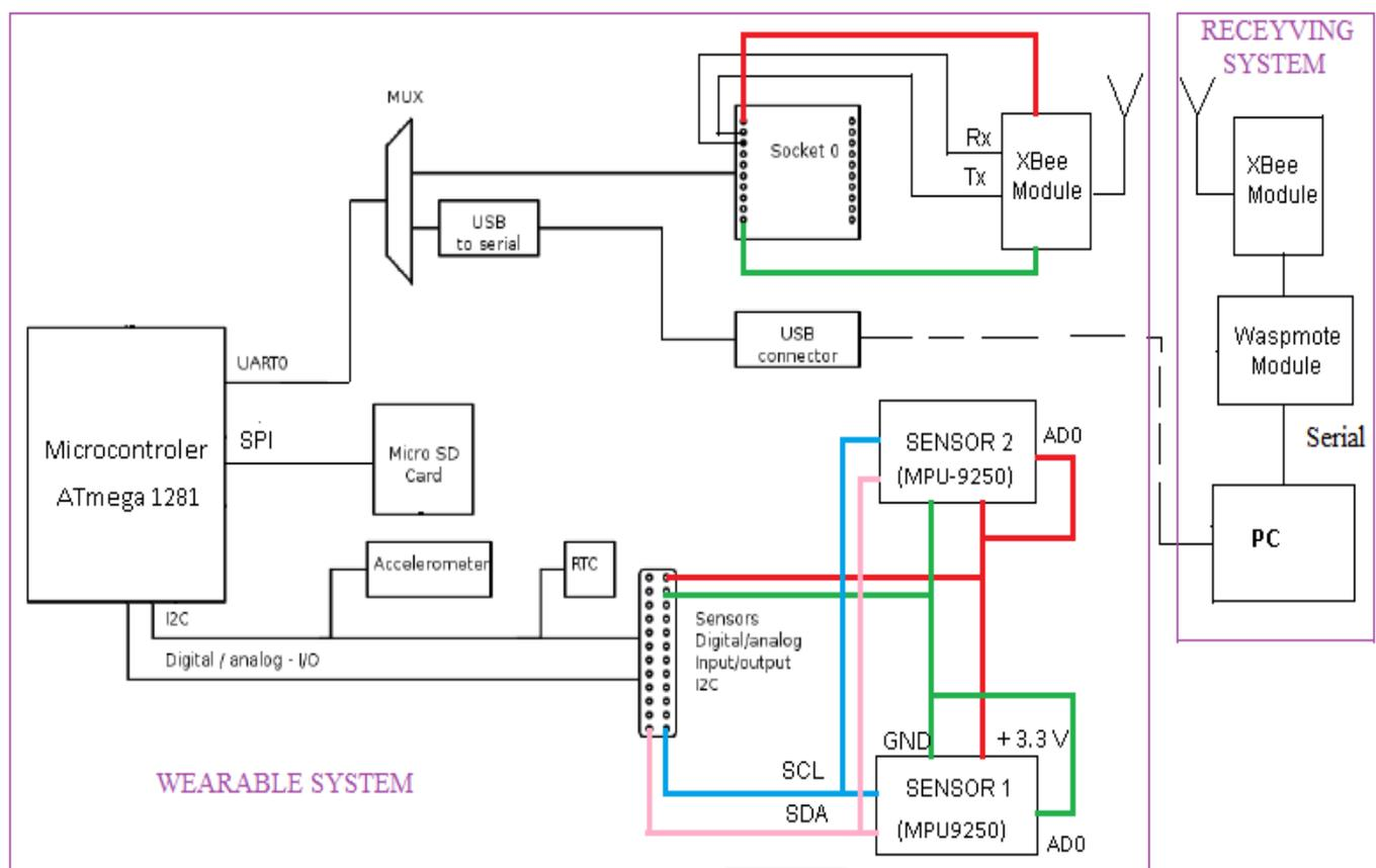
Fig.1. Data acquisition system using two inertial sensors
