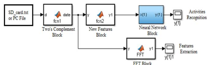
Fig. 5. Recognition system structure using System Generator [13]
