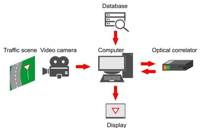
Fig. 1. Hardware scheme of Vertical Traffic Signs Detection System.
