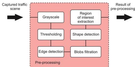
Fig. 2. Block diagram of pre-processing.
