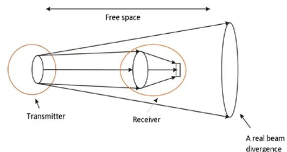
Fig. 1. Simple FSO architecture
