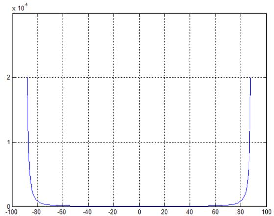
Fig. 2.  $CRB_{ULA}$  for  $K = 1$ ,  $SNR = 20 \text{ dB}$ ,  $\frac{d}{\lambda} = 0,5$ ,  $M = 16$ ,  $f = 2.4 \text{ GHz}$
