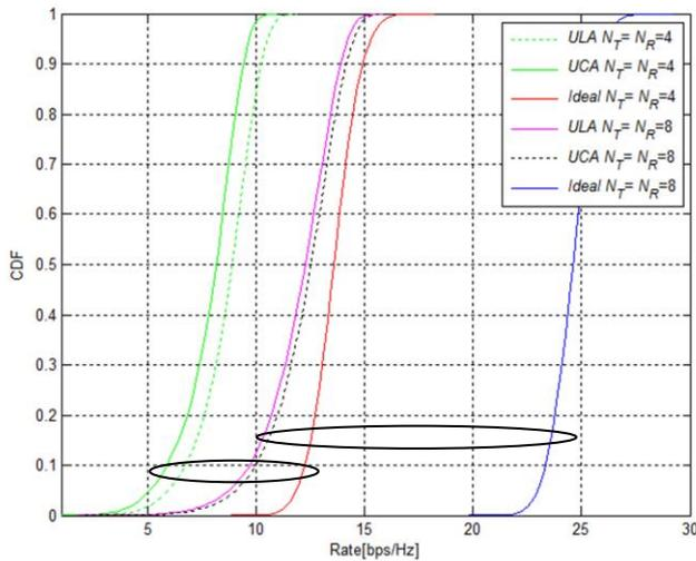
Fig. 3. Capacity CDF for different array configurations: ULA 4x4, UCA 4x4, ULA 8x8, and UCA 8x8. Mean SNR = 20dB.
