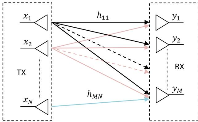
Fig. 1.  $N \times M$  MIMO channel matrix - complex coefficients  $h_{ji}$ .
