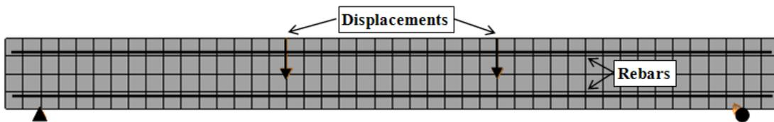
**Fig. 9.** Typical finite element mesh of numerical models.
