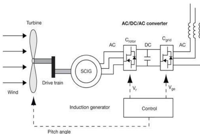
Fig-2 Fixed and variable speed WECS.
