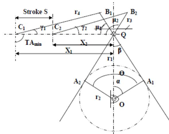
Fig.2 Limiting positions of the mechanism [12].
