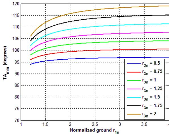
Fig.5 Minimum transmission angle of the mechanism.
