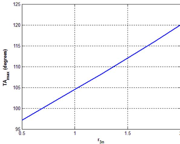
Fig.6 Maximum transmission angle of the mechanism.
