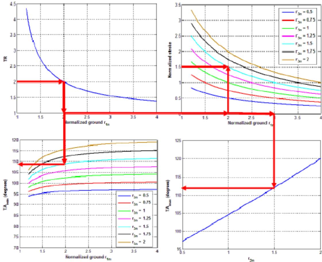
Fig.7 Synthesis nomogram of the mechanism.
