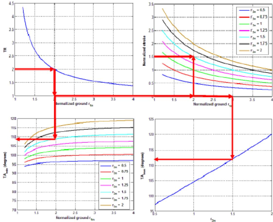
Fig.7 Synthesis nomogram of the mechanism.
