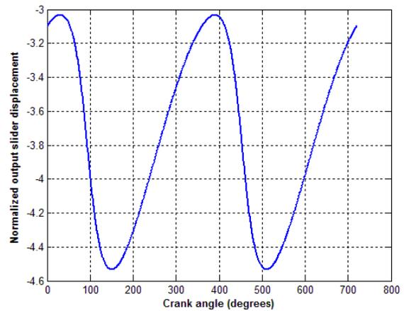
Fig.8 Normalized output slider displacement..
