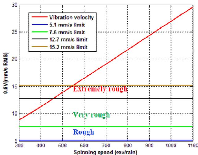
Fig.4 Vibration severity of the washing machine and Bernhard limits.
