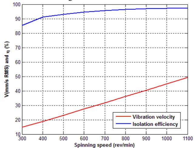
Fig.3 Optimal drum vibration velocity and isolation efficiency.
