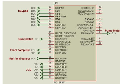
Fig.3 Pin Assignment of the Controller
