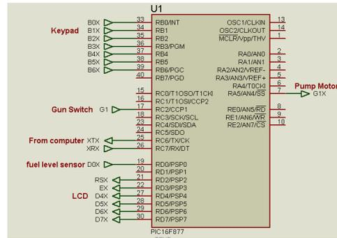
Fig.3 Pin Assignment of the Controller
