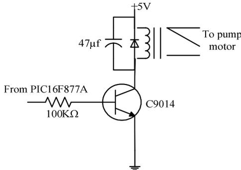
Fig.5 Circuit Diagram of Motor Driver
