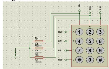
Fig.4 Key Pad Interfacing to Controller
