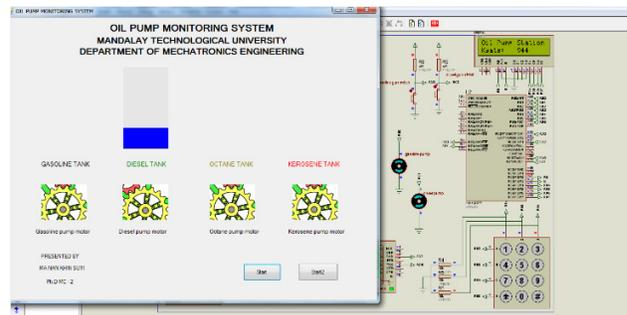
Fig.10 Simulation Result of Monitoring the Fuel Level from the Computer
