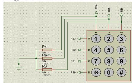
Fig.4 Key Pad Interfacing to Controller
