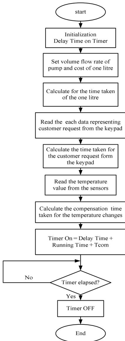
Fig.8 Time Control Flow Chart of the System
