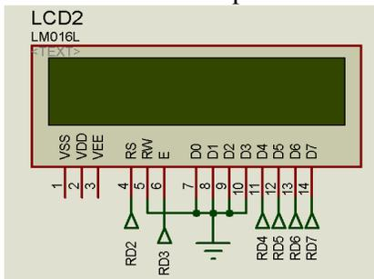
Fig.6 Pin Configuration between the LCD and PIC16F877A
