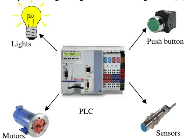
Fig.1. Typical functional components of PLC
