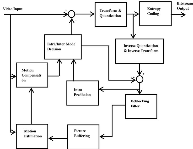
Fig. 2. Block diagram of H.264/AVC encoder
