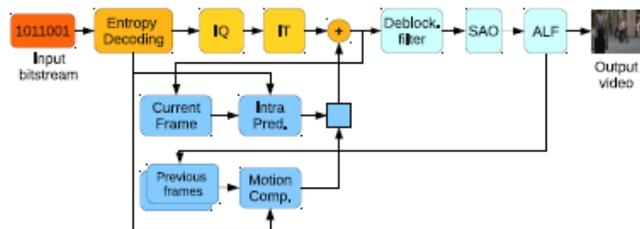
Fig.2 General diagram of HEVC Decoder [13]
