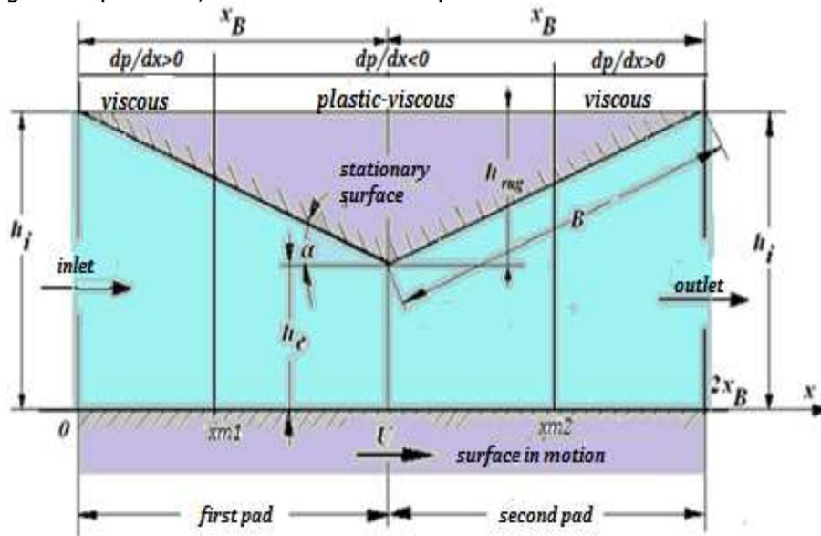
**Figure 1.** Roughness geometry proposed model, where the shear behavior areas are highlighted.
