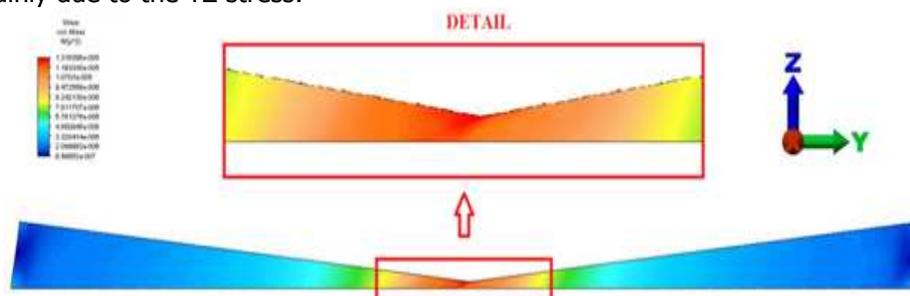
**Figure 3. Von Mises stress**
