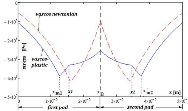
**Figure 2.** Maximum tangential shear stress along the lubricant film, in the case of occurrence of plastic shear
