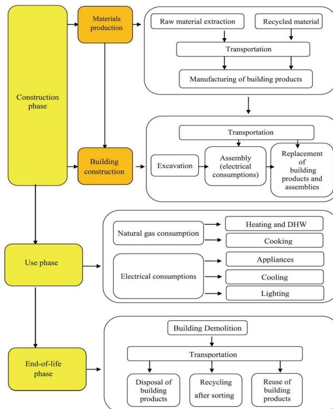
Figure 6: Suggested Framework of ECE-LCA Tool: All LCA Stages
