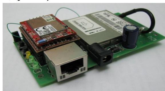
Fig. 8- WiPB prototype (dimension: 9.5cm x 5.5cm)
