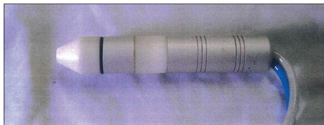
Figure 6: Hand piece of microdermabrasion unit
