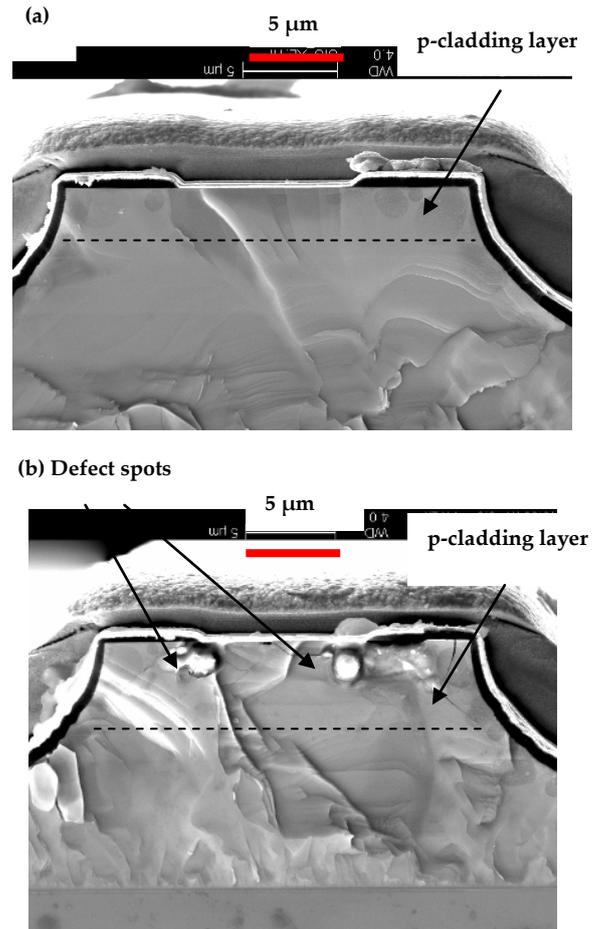
FIG. 5 (a) SEM PROFILE FOR LASER STRUCTURE, WHERE P-CLADDING REGION IS OVER THE DASH LINE. (b) TWO DEFECT SPOTS PRODUCED BY DRIVING CURRENT
