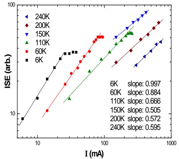
FIG. 4 THE INTEGRATED SPONTANEOUS EMISSION (ISE) AS FUNCTION OF INJECTED CURRENT AT DIFFERENT TEMPERATURES
