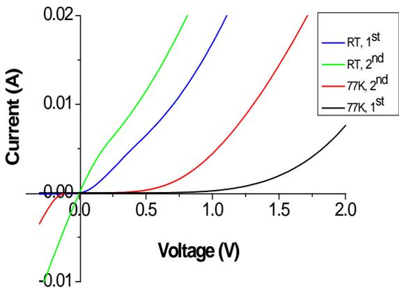
FIG. 3 CURRENT-VOLTAGE (I-V) CHARACTERISTICS BEFORE (1<sup>ST</sup> TEST) AND AFTER (2<sup>ND</sup> TEST) LASER DEGRADATION AT ROOM AND LOW (77K) TEMPERATURES
