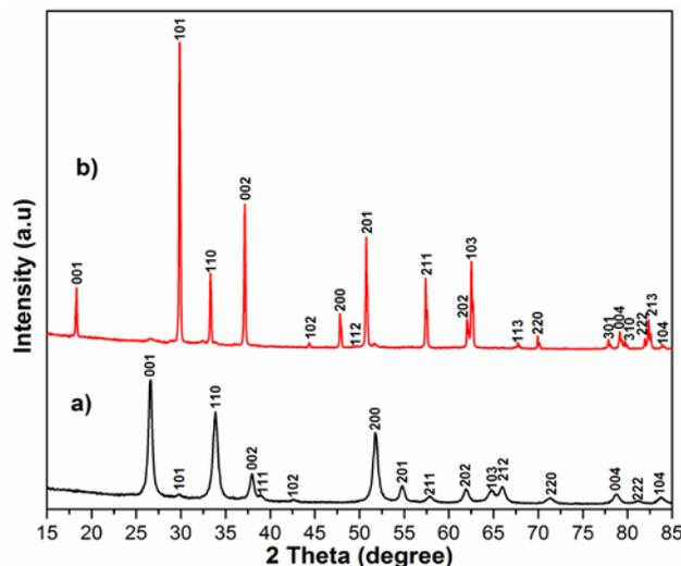
FIG. 3 XRD PATTERNS OF HYDROTHERMALLY PREPARED a) SnO<sub>2</sub> and b)SnO.
