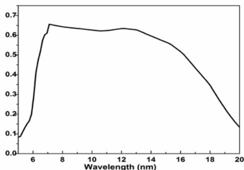
FIG. 3 The transmission spectrum of Zr filter.
