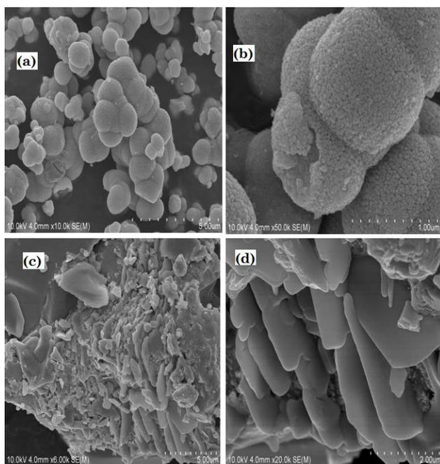
FIG. 1 FESEM IMAGES OF (a, b) SnO<sub>2</sub> SPHERES LIKE (c,d) SnO SHEET LIKE WITH DIFFERENT MAGNIFICATION RESPECTIVELY.
