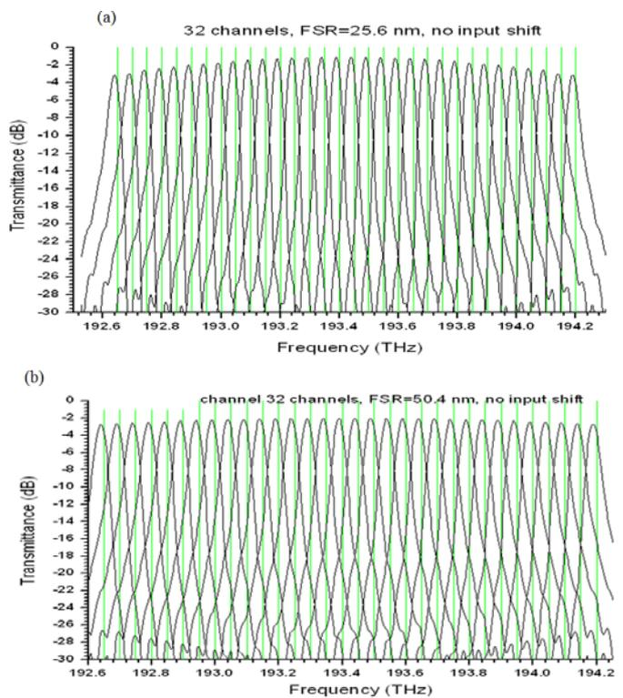
FIGURE 6: AWG TRANSMITTANCE MAPS: (a) FSR OF 25.6 NM, AND (b) FSR OF 50.4 NM, TOGETHER WITH THE INTERNATIONAL TELECOMMUNICATION UNION (ITU) GRID CHANNELS (50 GHZ SPACING) IN GREEN.
