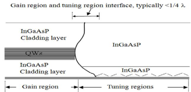
FIGURE 5: SCHEMATIC ILLUSTRATION OF A TYPICAL FABRICATED NARROW BAND TUNABLE LASER WITH AN UNDESIRABLE GAIN REGION AND TUNING REGION INTERFACE.
