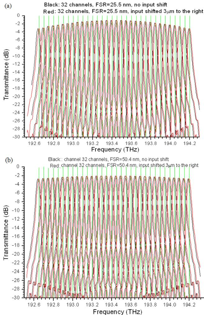
FIGURE 7: ADJUSTED AWG TRANSMITTANCE MAPS IN RED, WHICH ARE ALIGNED TO THE ITU GRID CHANNELS, BY SHIFTING THE INPUT WAVEGUIDE POSITION OF 3 NM TO THE RIGHT WITH REFERENCE TO ITS ORIGINAL CENTER POSITION: (a) FSR OF 25.6 NM, AND (b) FSR OF 50.4 NM, TOGETHER WITH THE INTERNATIONAL TELECOMMUNICATION UNION (ITU) GRID CHANNELS (50 GHZ SPACING) IN GREEN, AND THE UNADJUSTED AWG TRANSMITTANCE MAPS IN BLACK.
