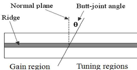
FIGURE 4: TOP VIEW OF THE INTERFACE ANGLE BETWEEN THE GAIN REGION AND THE TUNING REGIONS OF A NARROW BAND TUNABLE LASER.
