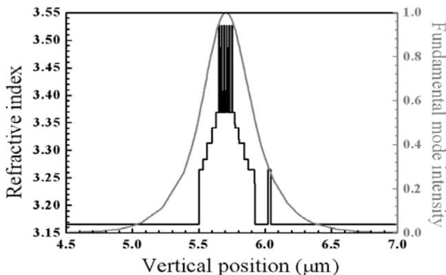
FIGURE 3: A TYPICAL OPTIMISED GAIN REGION: VERTICAL MODEL PROFILE AND REFRACTIVE INDEX PROFILE.
