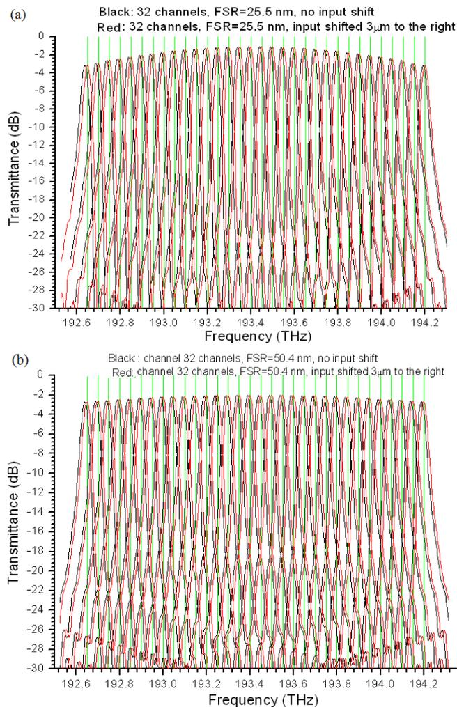
FIGURE 7: ADJUSTED AWG TRANSMITTANCE MAPS IN RED, WHICH ARE ALIGNED TO THE ITU GRID CHANNELS, BY SHIFTING THE INPUT WAVEGUIDE POSITION OF 3 μm TO THE RIGHT WITH REFERENCE TO ITS ORIGINAL CENTER POSITION: (a) FSR OF 25.6 nm, AND (b) FSR OF 50.4 nm, TOGETHER WITH THE INTERNATIONAL TELECOMMUNICATION UNION (ITU) GRID CHANNELS (50 GHz SPACING) IN GREEN, AND THE UNADJUSTED AWG TRANSMITTANCE MAPS IN BLACK.
