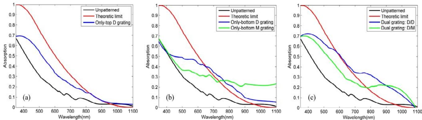
FIG.2 THE ABSORPTION SPECTRA FOR (A) ONLY-TOP GRATING, (B) ONLY-BOTTOM DIELECTRIC (D) OR METAL (M) GRATING, (C) DUAL GRATING OF TOP DIELECTRIC GRATING AND BOTTOM DIELECTRIC GRATING (D/D), AND OF TOP DIELECTRIC GRATING AND BOTTOM METALLIC GRATING (D/M). THE BLACK LINE IS THE ABSORPTION SPECTRUM OF UNPATTERNED SOLAR CELL. THE RED LINE IS THE THEORETIC LIMIT.
