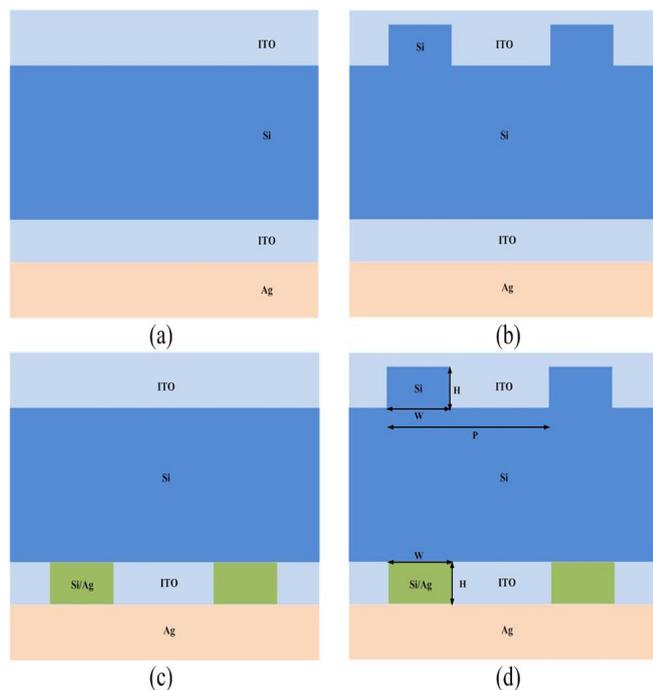
FIG.1 THE SCHEMATICS OF FOUR SIMULATED MODELS: (A) UNPATTERNED STRUCTURE. (B) ONLY-TOP GRATING. (C) ONLY-BOTTOM GRATING. (D) DUAL GRATING.
