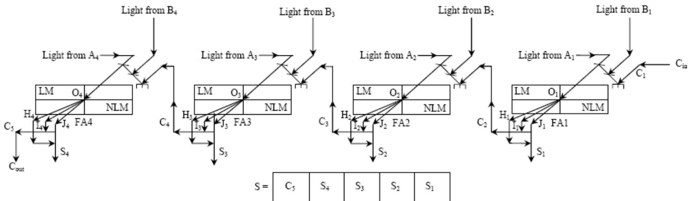
FIG. 7(B) ALL-OPTICAL 4 BIT PARALLEL ADDER CIRCUIT
