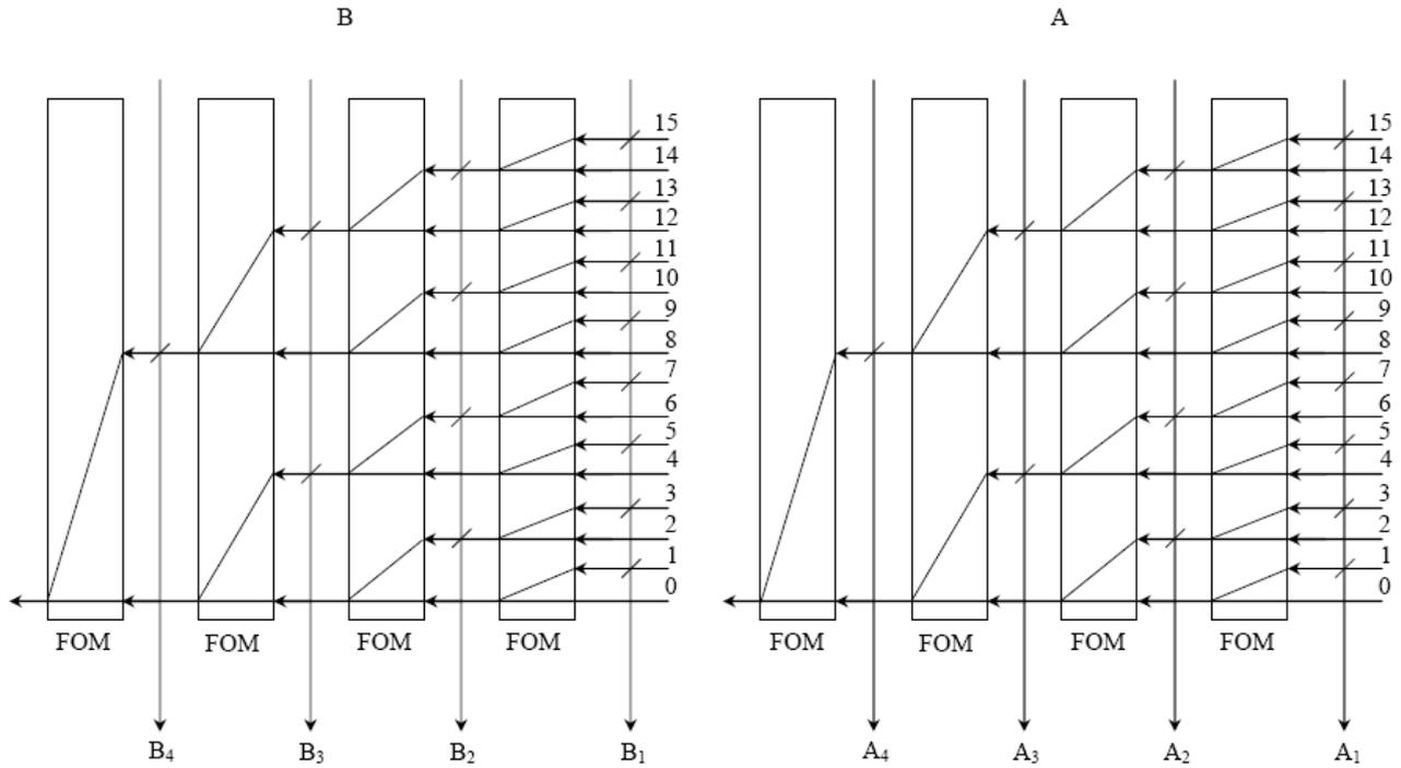
FIG. 7(A) ALL-OPTICAL DECIMAL TO BINARY CONVERTER AS INPUT TO 4 BIT PARALLEL ADDER CIRCUIT
