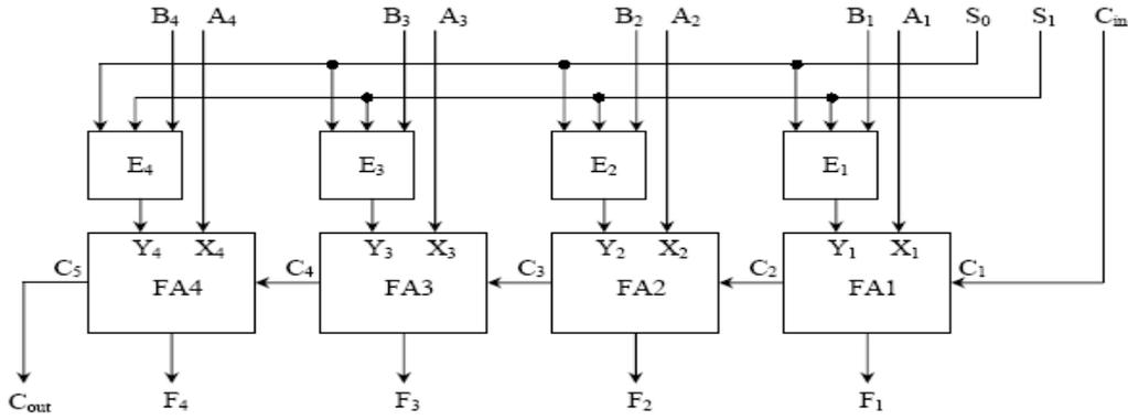
FIG. 4 ELECTRONICALLY ADDRESSED 4 BIT ARITHMETIC CIRCUIT
