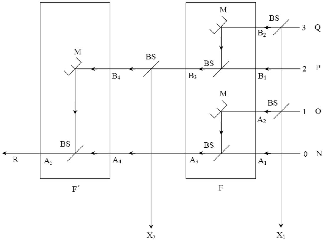
FIG. 5 OPTICAL TREE ARCHITECTURE
