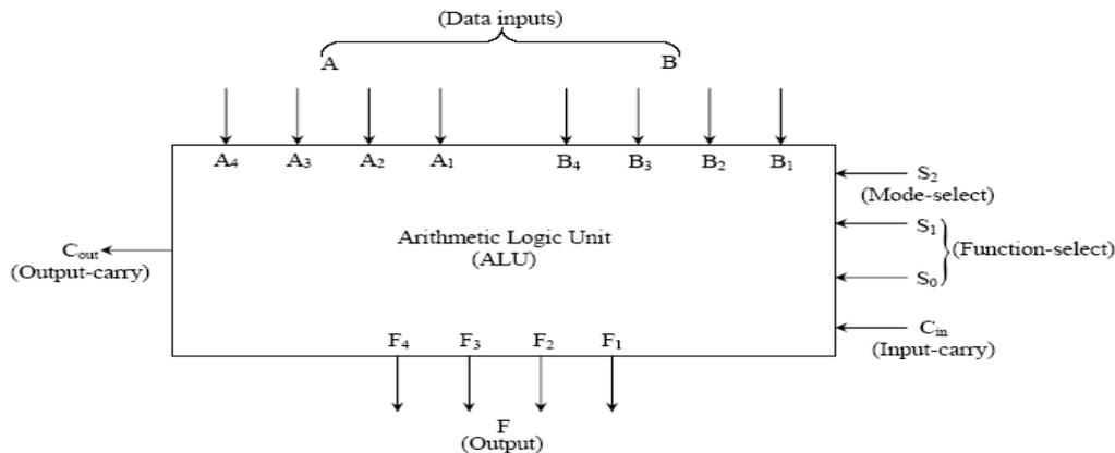
FIG. 3 BLOCK DIAGRAM OF A CONVENTIONAL FOUR-BIT ALU
