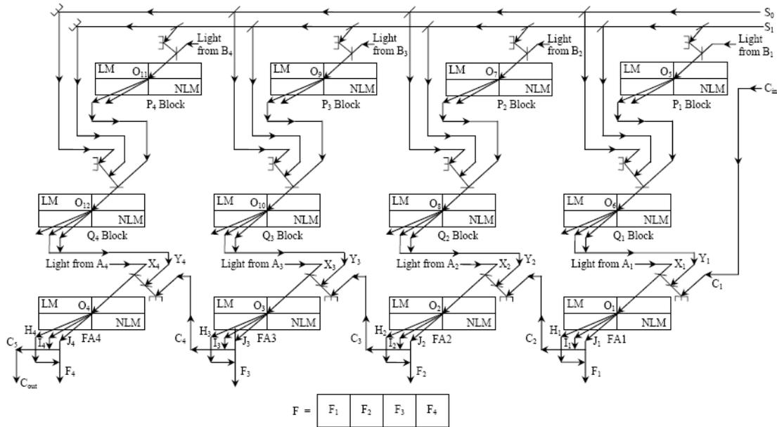
FIG. 9 ALL-OPTICAL 4 BIT ARITHMETIC CIRCUIT
