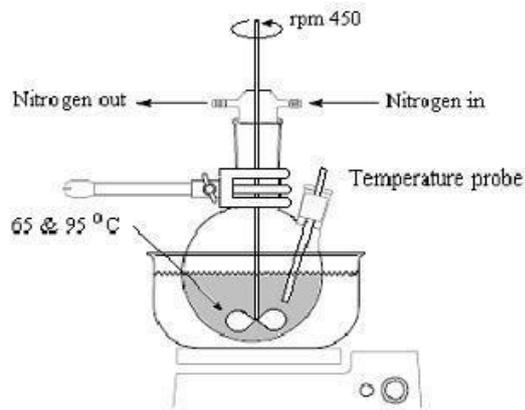
**Figure 1: Microsponges preparations by liquid-liquid Suspension polymerization**
