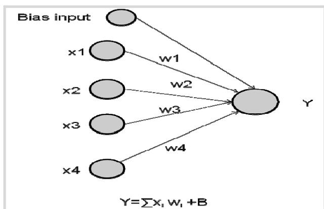
Figure 2: A simple feed-forward neural network
