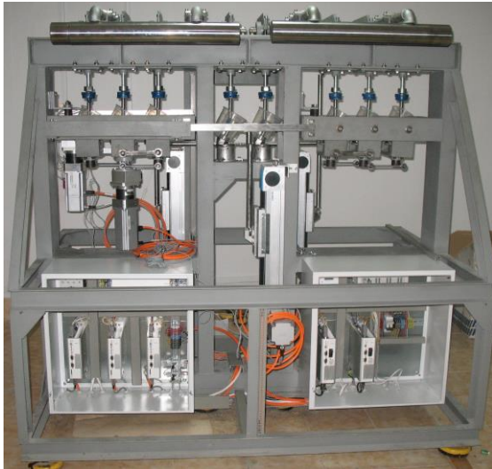
Fig.4. General view of the wear testing machine for total hip joint prostheses
